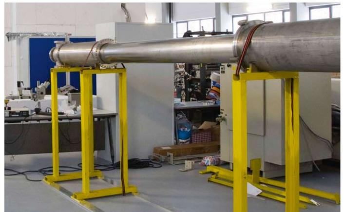
*Building of the experiment for the electric dipole moment in the neutron*
