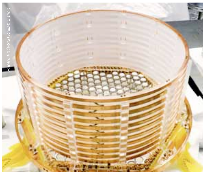
One half of the TPC in the clean room, during construction.
