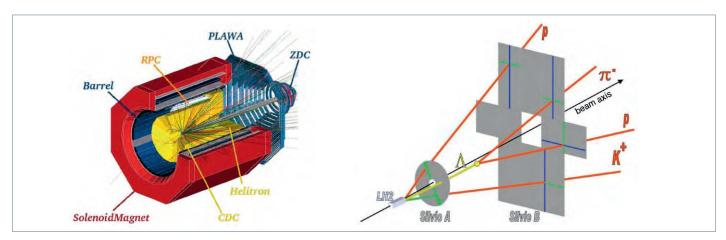
The image shows the FOPI detector (left). The SILVIO detector, designed and developed by L. Fabbietti's group is located inside FOPI.
