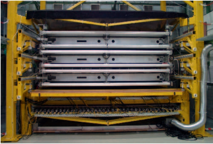
Measurement-setup for the calibration of the ATLAS muon chambers in Garching
