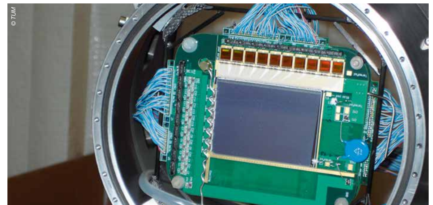
One of the experiment's four detector modules. The silicon module has been developed at the TUM. It detects about 10,000 particles per second.
